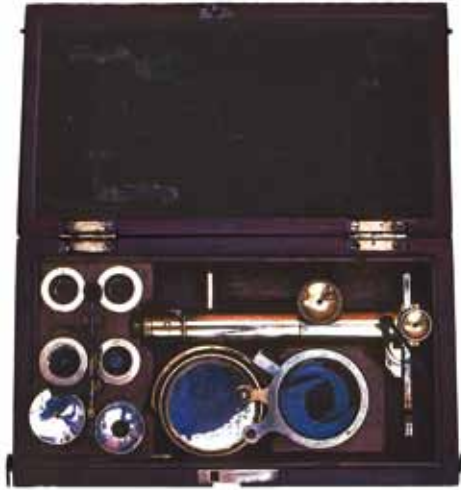
Fig. 4. The Linnean Society microscope packed in its case. Mahogany is used to make the case which is divided into sections and the lid of which is lined with bottle-green velvet. The main body and lens arm remain assembled during storage. Six lens holders (left) include two silvered Lieberkühn reflectors. The simple lenses magnify between 32.5x and 170x and provide remarkably clear images.
