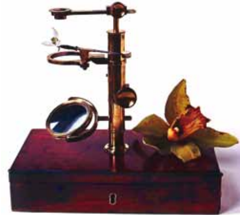
Fig. 2. Robert Brown's microscope at the Linnean Society with the stage forceps holding a specimen of the snowdrop Galanthus . The flower lying alongside is the orchid Cymbidium , for it was in the orchids that Brown first identified the cell nucleus. The focussing control (centre) is useful only for coarse adjustment. A cork insert within the cylindrical body supports the lens pillar (top) and allows fine focussing movements.
