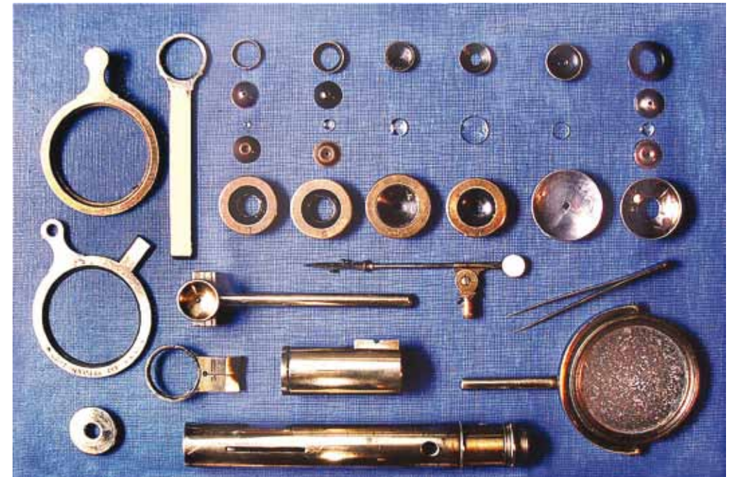
Fig. 7. Component parts of the Linnean Society microscope are here displayed in disassembled state. The stage assembly (left) and body components (below) can be identified. The six lenses (top) are held in place within the brass lens holders by retaining cups; and the aperture of the smaller lenses, being of higher power, were all restricted by means of perforated steel stops. Although this reduces resolution, it significantly increases image contrast.
