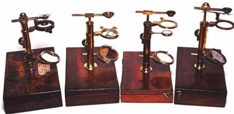
Fig. 1. Together after almost three centuries: four simple microscopes by Bancks, manufactured in London in the early 1800s. First is the Robert Brown microscope at Kew, fitted with fine focussing and bearing its commemorative silver plate. Next is that of Sir William Hooker, who used it in writing his Musci Exotici (1820), then George Bentham's microscope which still bears the tiny cutting marks from his plant dissections and, unusually, features a substage condenser lens. On the right is Brown's Linnean Society microscope.
