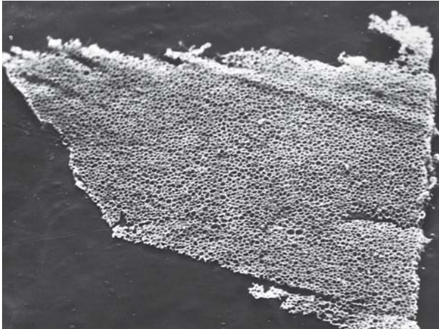
A Cambridge Stereoscan 600 SEM captured this image at low power of one of Leeuwenhoek's cork sections. Even by modern standards, this is an astonishingly regular and evenly cut section.
