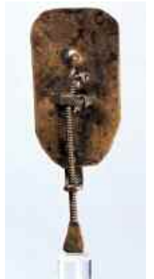
Utrecht University Museum holds this brass microscope, no bigger than a postage stamp, made by Leeuwenhoek. Unusually the lens is blown rather than being ground.
