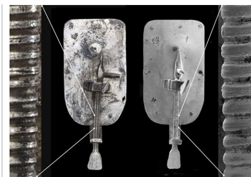
The recently discovered silver microscope under macrophotography at the Christie's studio (left) compared with the finished SEM study (right). Details of the main screw just visible to the naked eye can be discerned with diagnostic clarity under the high-resolution SEM image.
