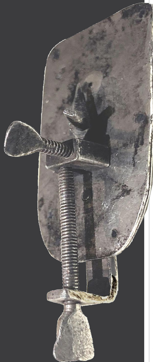
A house clearance in East Anglia in December 2023 revealed this little microscope which proved to be hand-made by the Dutch pioneer Leeuwenhoek some 350 years ago. The main screw was used to set the specimen at the desired height; a silver pin held it close to the single lens.
