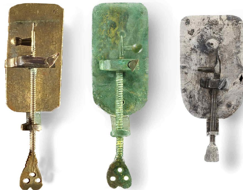
LEFT Replica Leeuwenhoek microscope of brass sold by the Boerhaave Museum, Leiden. It is a faithful copy of an authenticated instrument in their collections.
