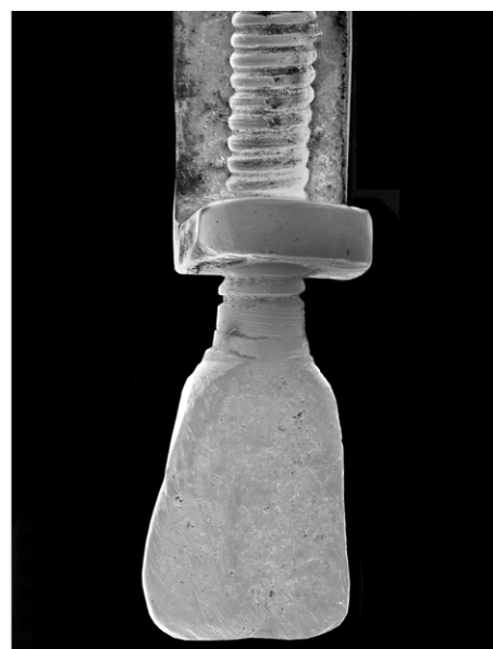
RIGHT Leeuwenhoek needed the construction of his microscopes to be functional, rather than precise. The silver handle was beaten to shape, with little attempt to make it symmetrical.
